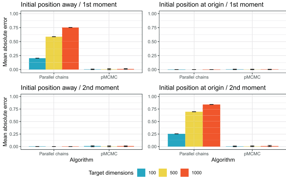
FIG. 2. Means and 95% confidence intervals for mean absolute estimation error from 10k parallel MH chains versus a single parallel MCMC chain produced by Algorithm 4 using 100k proposals. Both target isotropic Gaussians of 100, 500 and 1000 dimensions using 10k MCMC iterations. Estimator from 10k parallel chains demonstrates adverse dependence on starting point: starting at distribution mean \mathbf{0} harms second moment estimator, but starting at \mathbf{1} harms first moment estimator. The difference between chain and proposal counts arises from memory constraints on the multi-chain approach and does not appreciably change results.
